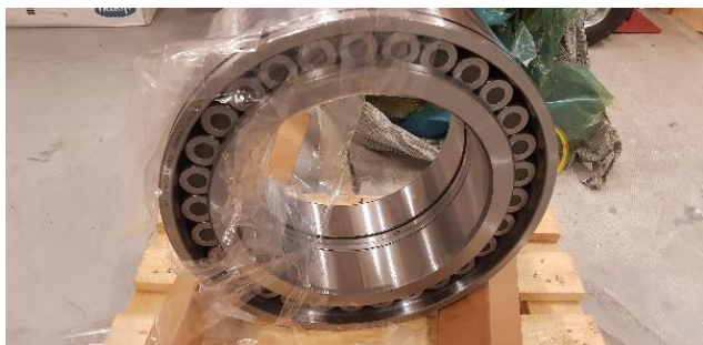
Roller bearing before installation of offshore seals
